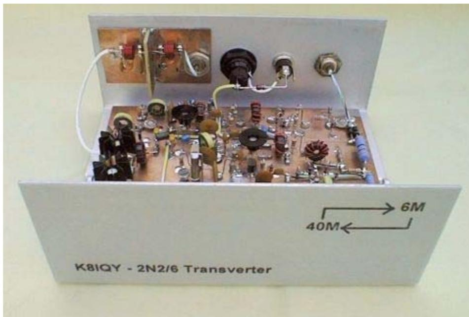
This project is a 40 meter to 6 meter CW "no tune" transverter using ten 2N2222 transistors and one 2N2907. The transverter requires 2 watts of drive from a 40 meter cw transceiver and outputs 2 watts on 6 meters. On receive, it uses the 40 meter rig as the intermediate frequency amplifier. Its receive sensitivity is approximately 0.5 microvolts. Transmit spurious outputs are less than -50 dBc, meeting FCC spectral purity at a 2 watt power level. All transmit/receive switching is solid state.
